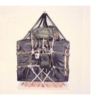
The A-22 loads can be rigged for low-velocity drops
