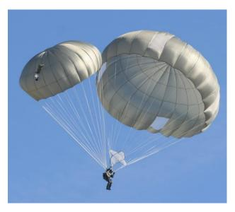
The C400 Main Assembly (C400M) consists in a polyconic canopy 45-foot nominal diameter built in 24 gores of 0.5-3 CFM rip-stop, orientable through control toggles, without valve in the apex nor anti-inversion net in the leading edge, Dacron independent suspension lines, 4 symmetrically positioned stabilization windows and slider, which allows the use up to 150 Knots with a descent speed of 4.92 m/s with 185 kg suspended weight.
