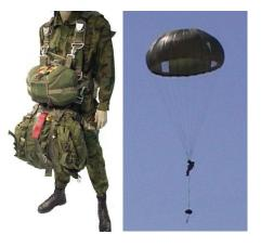
The H-Harness consists of two equipment retainer straps and it is used to rig the rucksack or any other operational load/weapon to the parachute harness. Two adjustable leg straps are provided to secure the pack to the parachutist's legs. The leg straps are equipped with the male portion of the leg strap release assembly.
