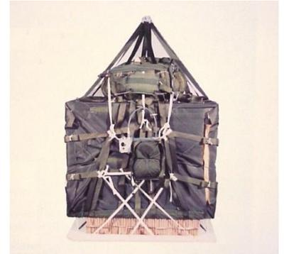
The A-22 loads can be rigged for low-velocity drops with one G-12E as primary parachute for 501 to 2,200 pounds suspension weight. As alternate parachute can be used a G-14 in two cluster for 501 to 1,000 pounds and three cluster for 1,001 to 1,500 pounds.
