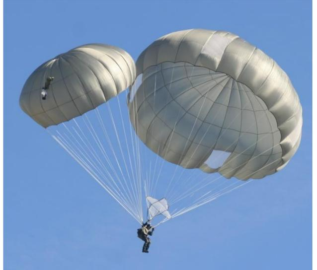
The C400 Main Assembly (C400M) consists in a polyconic canopy 45-foot nominal diameter built in 24 gores of 0.5-3 CFM rip-stop, orientable through control toggles, without valve in the apex nor anti-inversion net in the leading edge, Dacron independent suspension lines, 4 symmetrically positioned stabilization windows and slider, which allows the use up to 150 Knots with a descent speed of 4.92 m/s with 185 kg suspended weight.
