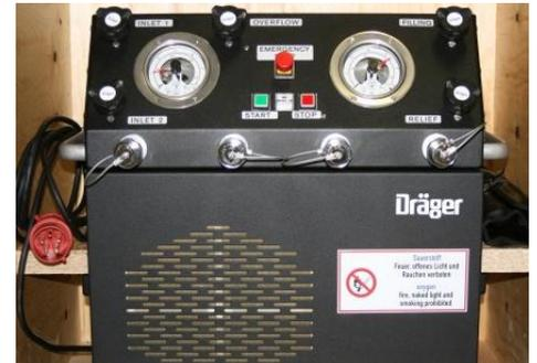
**OXYGEN BOOSTER DOB-H (P/N 6531300)** is a mobile manually operated pump to charge the oxygen cylinders in the field.
