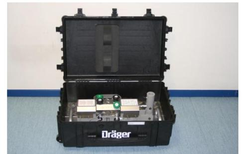
**MOBILE OXYGEN TESTER (P/N E34500-01)** has been developed as a field tester for the OXYJUMP system to enable that the equipment can be tested before and after each mission.
